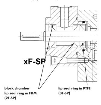
Standard inlet pressure p1: 7 bar (in certain special solutions up to 50 bar!) Before start-up the block chamber must be filled with fluid. **Beinlich Pumps** recommends using Mesamoll® oil or another inert medium which does not react with the pumped fluid and which is environmentally inert should it leak.
