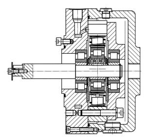
The magnetic coupling must be bleeded by the flange.
